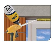
Tekapur Standard gun grade is a one-component polyurethane foam to be used with a gun. It is hardened by air humidity.
